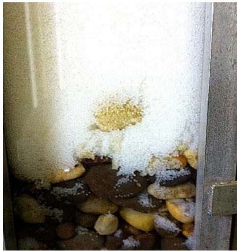
Fig. 10. Particles adhered to PS grains that sediment during the backwashing process, when the water's superficial velocity was 6.6 m/h (0.11 m/min).
