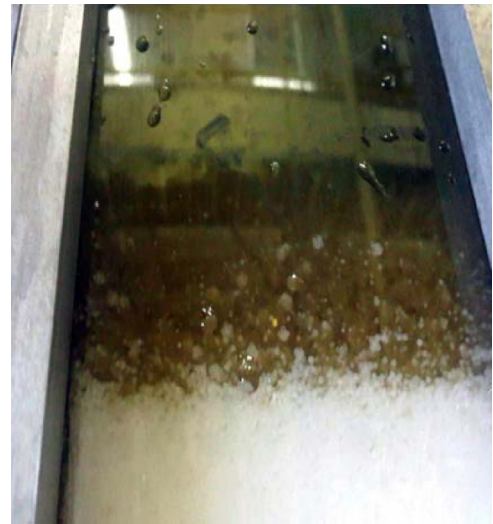
Fig. 11. Segregated particles and PS grains with an ascension velocity of 6.6 m/h (0.11 m/min) when the drag force was insufficient.
